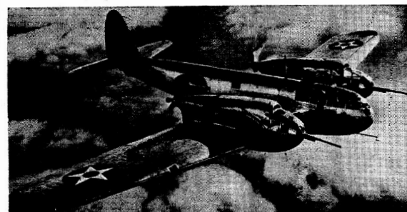
One of the new "Airacuda" fighting planes of which 13 have been ordered by the War department. The plane, of revolutionary new design, has a lighting outline above 30,000 feet, has its propellers located behind the wings instead of in front and is equipped with two specially designed engines. The War department states that the speed of the plane "is believed to be sufficient to overhaul any modern bomber now in production or building."
