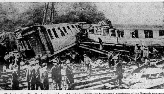
Made shortly after the tragic accident, this photo shows the telescoped carriages of the French passenger express in which 27 persons were killed when the train jumped the rails near Villeneuve St. Georges. Rail-road officials attributed the accident to faulty setting of a switch.
