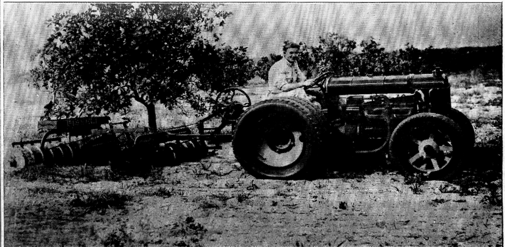
The above illustration shows the latest equipment for tractors. The rubber wheels give traction in loose sand.
