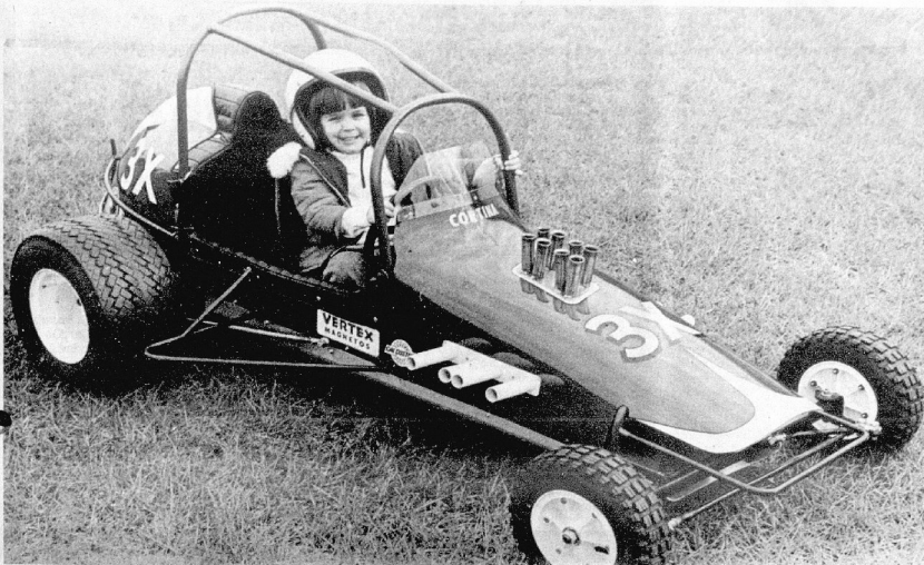
COMPLETE WITH AIR intake stacks, electric brakes and centrifugal clutch,
