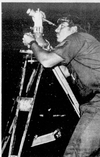
USING A THEODOLITE S. Sgt. Mike Szykowski gets the instrument in alignment to measure the angle between his location and Polaris the North Star. He is one of only a few men able to keep both eyes open while using the theodolite. Recording the readings and time is Airman Charles Lemarie who normally is seated in the lighted van where he can read the chronometer. Photo—Miller.
