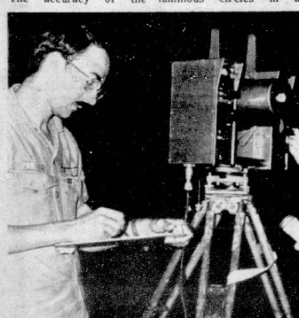
PART OF A four man geodetic survey team T. Sgt. James Baxley adjusted the geodimeter before taking a reading on a target about 1.2 miles away on Memorial Highway.
