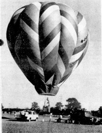
AFTER BEING PARTIALLY filled with air the huge balloon gains buoyancy by being filled with heated air from a butane burner. Airborne Steve Roberts starts on his way towards the Avon Park airport. Photo — Miller
