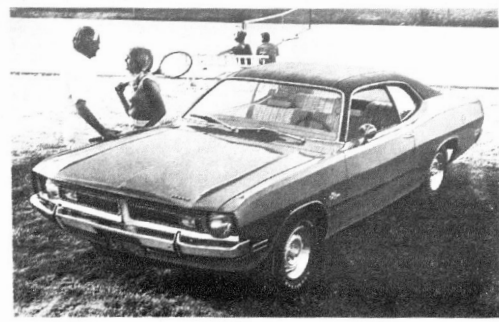
DEMON FOR ECONOMY — New addition to the Dodge compact line for 1971 is the 108-inch-wheelbase Demon, which combines economy and sporty look. Engines range from the 198-cubic-inch Slant Six to the 340-V-8.
