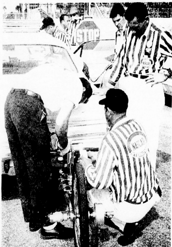
The fifth wheel. All entrants in the Trials are fitted with the special wheel (above) for more accurate recording of speed and distance traveled. Cables lead to instruments inside the car (below) where graphic records are produced.
